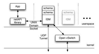
Figure 9: Omega prototype implementation, end host view with an application and ISM in use. UDP encapsulation of traffic is used in PlanetLab tests, whereas Open vSwitch is used with our IPv6 variant. The grayed ISM highlights the fact that multiple ISM daemons co-exist and have their own appropriate schemas.
