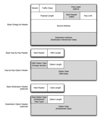
Figure 10: Structure of the Omega-v6 header. Shaded fields represent re-use of IPv6 fields for encoding of Omega values.
