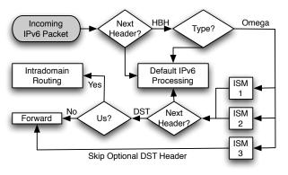
Figure 11: Packet processing by our Omega-v6 Open vSwitch router.
