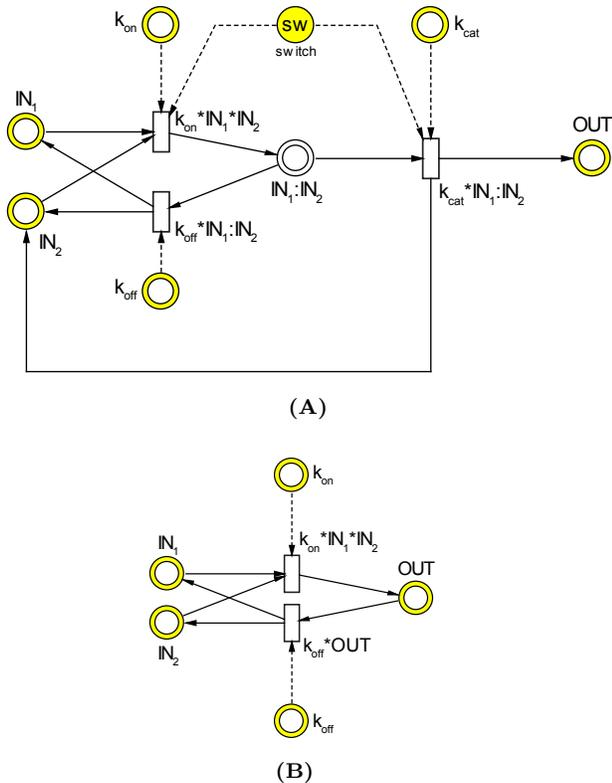
**Figure 1: Continuous time/state Petri net modules.** (A) The activation module, which models the activation of a zymogen ( $IN_1$ ) into its active configuration ( $OUT$ ) by a catalyst ( $IN_2$ ). In versions with the discrete switch  $sw$ , the module is hybrid, and models the switching on/off of a reaction by the presence/absence of a variable. (B) The binding module, which models the (reversible) binding of two components,  $IN_1$  and  $IN_2$ , into the macromolecule  $OUT$ .
