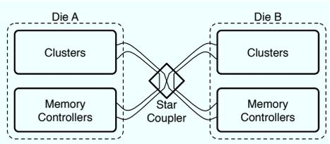
Figure 2: Logical view of a two die system
