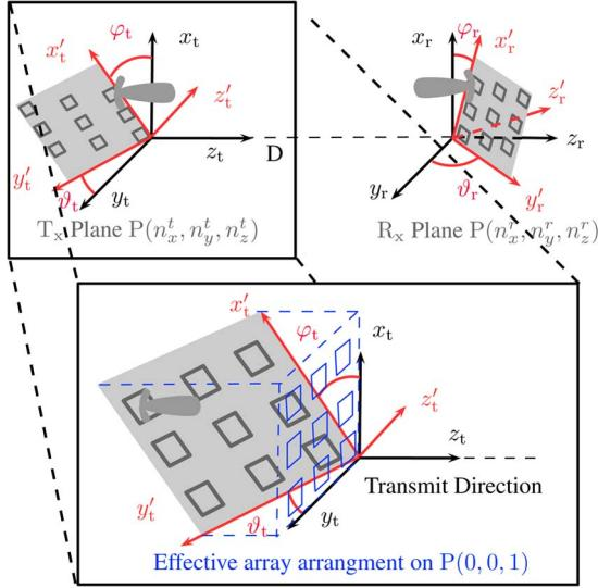
Fig. 3. Oblique UPA. Two parallel Cartesian coordinate systems are located at  $T_x$  and  $R_x$  with origins at the bottom right of the  $T_x$  UPA and bottom left of the  $R_x$  UPA. The  $z$ -axes are both in direction from  $T_x$  to  $R_x$ .
