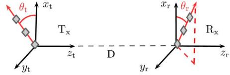
Fig. 2. Oblique ULA. Two parallel Cartesian coordinate systems are located at  $T_x$  and  $R_x$  with origins at the lower ends of the ULA. The  $z$ -axes are both in direction from  $T_x$  to  $R_x$ . The  $T_x$  array is located in the  $xz$ -plane.
