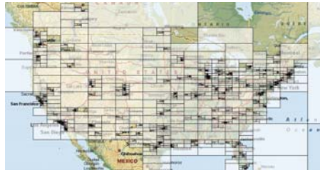
Figure 4: The structure of the PHT for the 1.4 million input data set and a block size of 1000.
