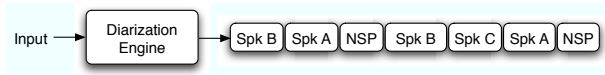
Figure 1: The output of a speaker diarization system separates the input stream by speaker and non-speech (NSP).
