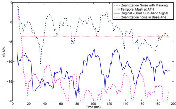
**Fig. 2.** Application of temporal masking to reduce the bits for 200ms region of a low energy sub-band signal. The figure shows a portion of sub-band signal, temporal masking threshold for that region, quantization noise for the base-line codec and for the codec with temporal masking.
