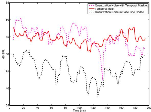
**Fig. 3.** Application of temporal masking to reduce the bits for 200ms region of a high energy sub-band signal. The figure shows the temporal masking threshold for a high-energy region of sub-band signal, quantization noise for the base-line codec and for the codec with temporal masking.
