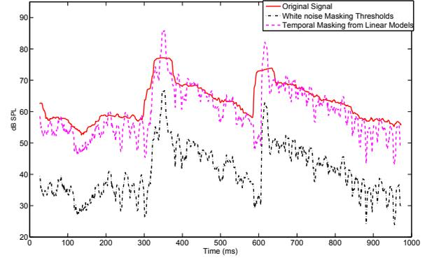
Fig. 1. Example of 1000 ms sub-band signal in dB SPL, the linear masking model and white noise masking thresholds.
