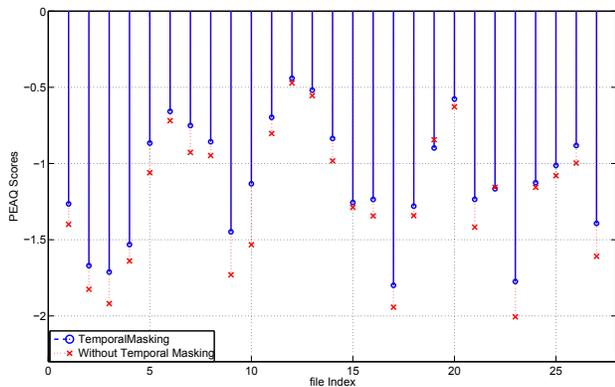
**Fig. 4.** Comparison of PEAQ scores for codecs at the same bit-rate for the files in the data-base; a fixed bit-rate FDLP codec versus variable bit-rate FDLP codec utilizing temporal masking.
