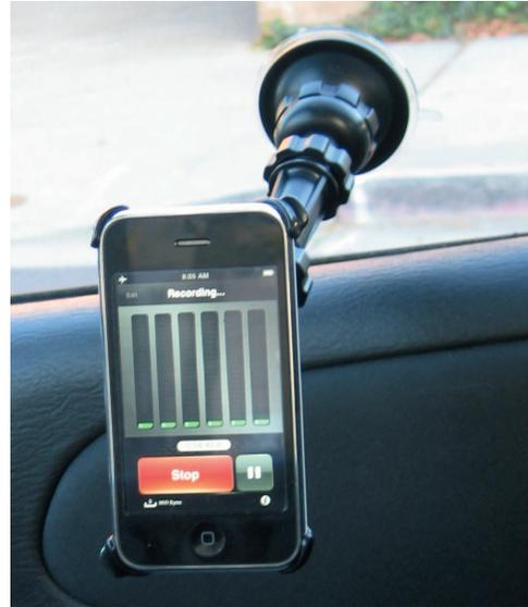
**Figure 1. An iPhone mounted to the car windshield running the program “Recorder” was used to record the noise and car conversations, simulating a built-in microphone in the car.**
