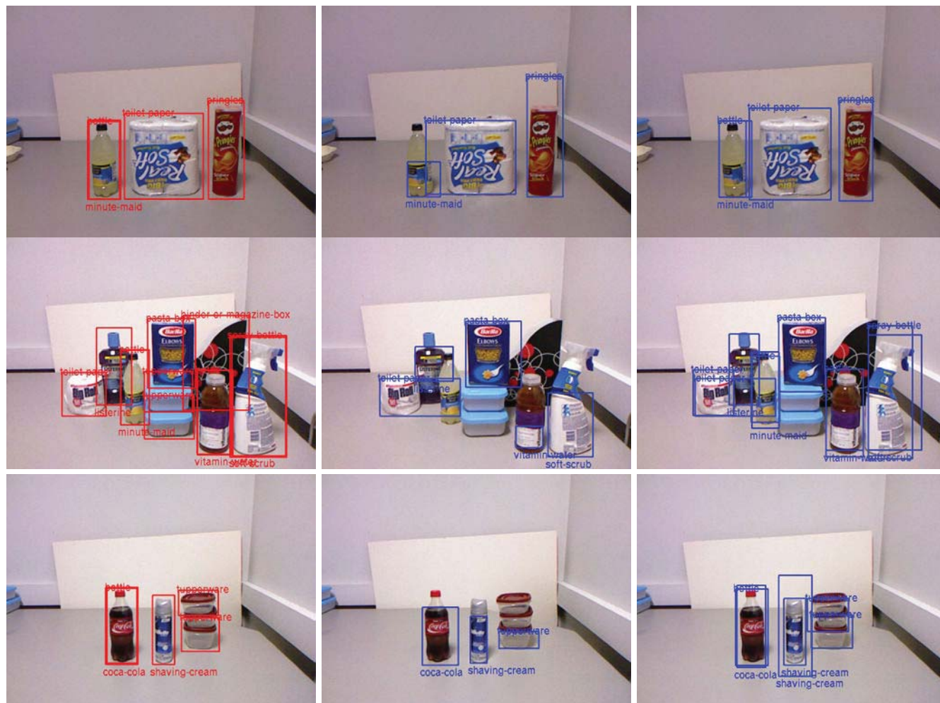
Fig. 6: Each row shows sample detections on a test scene. From left to right: (1) human annotations, (2) local feature NBNN ( LF ), (3) our method.
