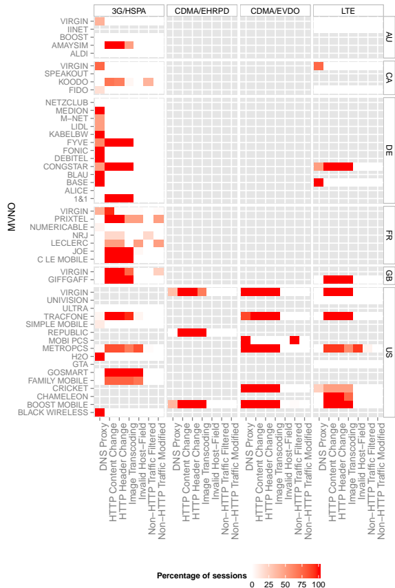
Figure 6: Deployment and behavior of DNS and HTTP proxies for the MVNOs in the considered countries. Only TracFone and Cricket in the USA, and Virgin and Numericable in France, are full MVNOs. The rest are light MVNOs.
