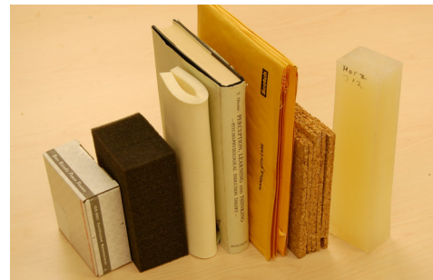
Fig. 6. The final test set. In order from left to right: Cardboard Box, Dark Foam, Light Foam, Hardcover Book, Cushioned Envelope, Layered Cork, and Rough/Smooth Acrylic (different sides of the same object).
